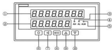
Table with 2 columns: 名称, 说明. Lists display windows (total and differential accumulation), indicator lights (control and alarm), and operation keys (set, left, confirm, increase, decrease).
