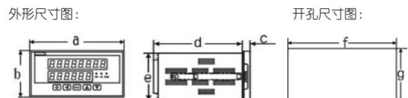
Table with 8 columns: 规格, a (mm), b (mm), c (mm), d (mm), e (mm), f (mm), g (mm). Row 1: 160x80, 160, 80, 10, 115, 75, 152.1, 76.1
